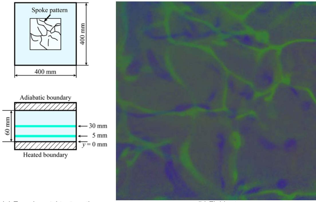
(a) Experimental test section
